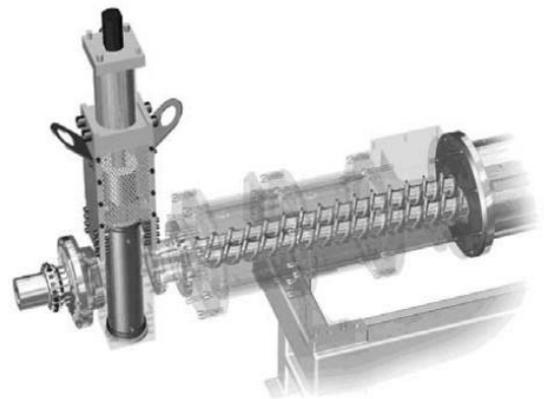
The C<sup>2</sup>TX's conical design allows for positive compression in the barrel and reduces possibility of back feeding. Positive compression yields an efficient manner of imparting mechanical energy into the extrudate. The conical design of the C<sup>2</sup>TX causes the material to be kneaded and sheared along the screw profile. In traditional twin-screw extruders, the melt is kneaded and sheared by shear
