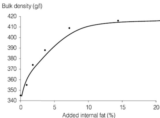
Nutritional requirements dictate the levels of total fat required in most feeds. The total fat levels can vary from 3% to greater than 40% in some aquatic feed diets. As the fat level increases, there is an expected increase in the bulk density of the feed. In one study conducted at the Wenger Technical Center, an aquatic diet containing 60% fishmeal,
