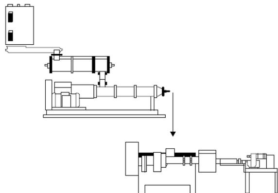
This processing system has the advantage of being able to operate both extruders at their maximum rate potential. When only one extruder is used to produce a very dense pellet, the extruder may have to be operated at lower throughputs to prevent expansion. Adding the second forming extruder (PDU) can allow a feed manufacturer to produce a
