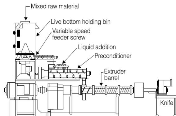
Each component is designed to accomplish a specific function in the process of cooking and forming feed products. The operating conditions can be adjusted to vary the characteristics of the finished product.
